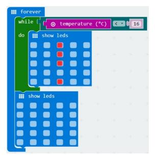
4.3. The program is finished. Now test it. First of all, test it virtually - change the temperature so that it would be lower than 16:
