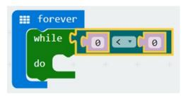
Micro: Bit evaluates illumination in numbers from 0 to 255. You need to compare the current illumination with a predetermined low light level (for example, 50).
