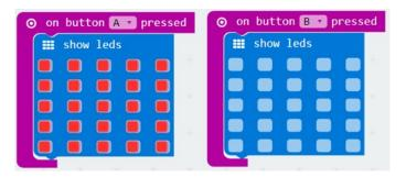
2. Test the program again. After pressing the button "A" (in the results field), the lights have to turn on and when you press "B" – they should be turned off.
